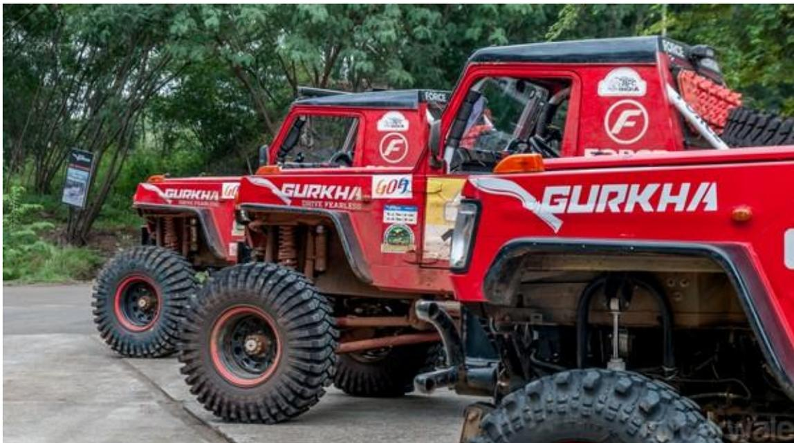
Surprisingly, the brutal diesel engine noise is produced by a stock 2.2-litre four-cylinder mill that produces 140bhp/320Nm of torque and is the same one found in the Force One SUV. The package includes a five-speed manual and locking differentials to make it a fully capable off-roading vehicle. There is a noticeable whistle when the driver gets off the accelerator and there is a snorkel intake to aid with the water wading capabilities.
