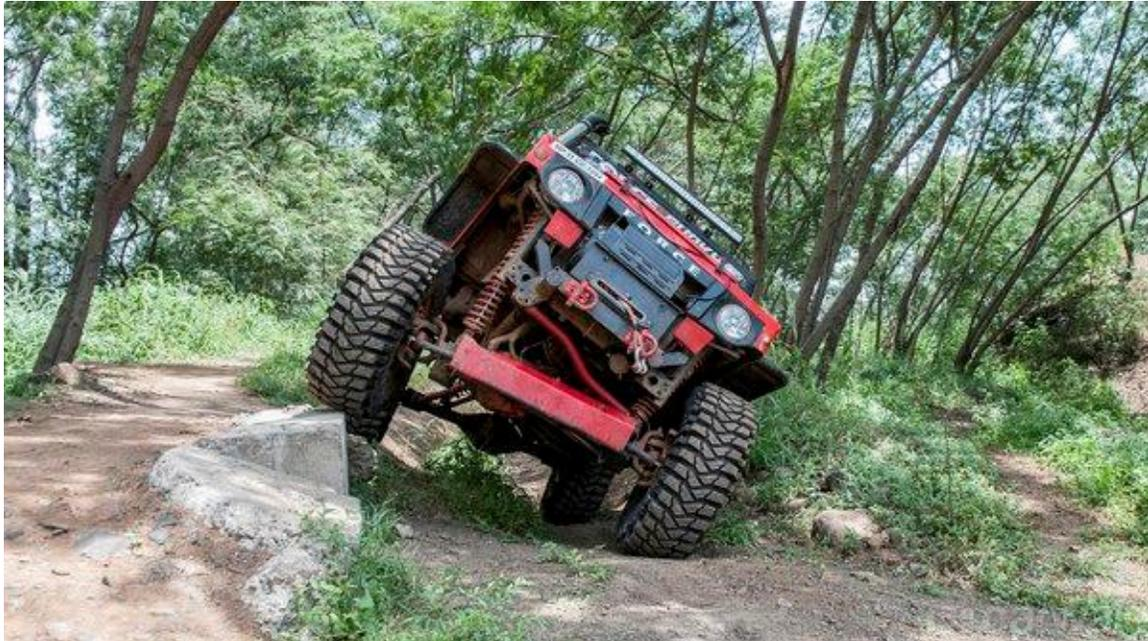
Sounds complicated? Well, I thought so too and so discovered that the best way to convey what these changes meant to the vehicle was by giving you an idea of its increased capabilities. It can now scale a gradient with a 60-degree incline as compared to the previous RFC Gurkha's 45 degrees. The approach and departure angle have increased from 50/44 to 88/58 respectively. Finally, the water wading capability has also gone up from 1000mm to 1100mm.
