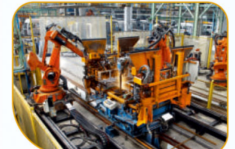
Robotic Welding - made entirely of pressed steel panels
