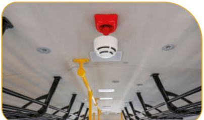
Factory fitted concealed FAPS - Integrated and concealed, factory fitted fire safety system for complete peace of mind. Ensures protection while maintaining a clutter-free and comfortable cabin
