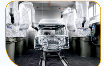
Robotic Painting for car-like gloss and even Paint finish
