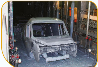
7th Gen CED Dip Painting Process - provides anti-rust protection
