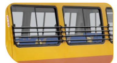
Window railings for additional safety
