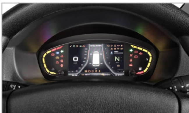
All New TFT Digital Instrument Cluster with Vibrant Graphics, at-a-glance Readability, Gear Indicator, TPMS, Door-open Alerts & Tell-tale Indicators
